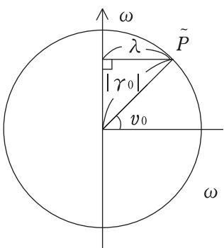
$$\begin{aligned} \lambda &= |\gamma_0| \cos v_0 \text{だから} \\ \frac{d^2\gamma_0}{dt^2} &= \omega^2 \lambda = \omega^2 \gamma_0 \cos v_0 \\ \text{ここで } \gamma_0 &= 6378 \text{ km} \\ \text{地球の角速度 } \omega \text{ は} \\ \omega &= \frac{2\pi}{23.94(h)} = 6.28 \div 86184(s) \\ &= 7.290 \times 10^{-5}(\text{rad/s}) \end{aligned}$$
